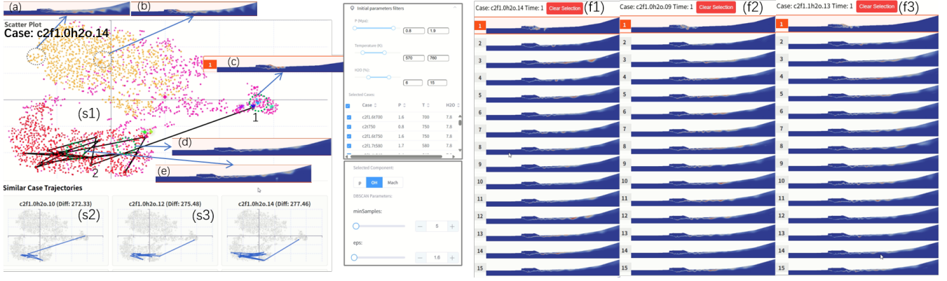
Figure 8: Case Study 2: Clustering of OH Field Trajectories to Identify Combustion Modes. The temporal trajectory of the selected case was shown in region (s1), with its two most similar trajectories located at (s2) and (s3). The corresponding OH field images for these cases were displayed in (f1)–(f3). Two distinct combustion modes were identified: the red cluster corresponds to the shear layer combustion mode , characterized by narrow, stratified flame structures along the fuel–air interface (see circled regions in (d)–(e)); the yellow cluster corresponded to the jet-wake combustion mode , where the flame formed a wide, curved tail extending from the fuel inlet (see circled regions in (a)–(b)). The clustering results demonstrated that the system could effectively separate and characterize combustion behaviors across different cases, even when OH field trajectories fluctuated at steady state.
